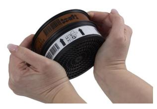
**1.2** Place the particle filter on top of the cartridge. Grasp both protective elements. Squeeze hard until you hear the particle filter snap onto the gas filter.
