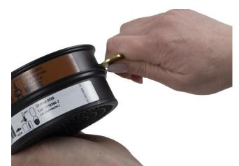
1.4 To separate a combined filter, place a coin it in the space between the lower lip of the particle filter and the small tab molded into the side of the gas filter. Push firmly and twist the coin until the filter pops off.
