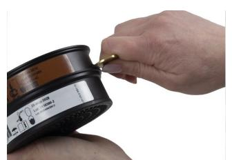
**1.4** Place a coin it in the space between the lower lip of the particle filter and the small tab molded into the side of the gas filter. Push firmly and twist the coin until the filter pops off.
