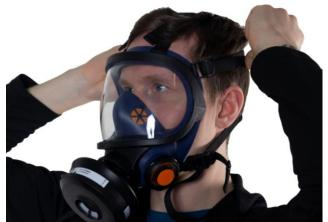
4.4 Tension the elastic straps in pairs by pulling the free strap ends towards the rear. Adjust the fit of the mask on your face, so that it fits firmly but comfortably. Adjust the lengths of the upper pair of straps and fix by means of the buckles.
