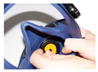
**7.1** One membrane is in the center of the inner mask on a fixed dowel. Prise off the membrane and fit a new membrane.
