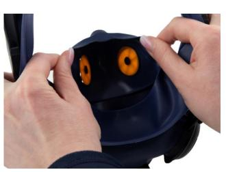
7.2 Two membranes are fitted, i.e. one on each inside of the inner mask. The dowels for these membranes are removable and should be changed whenever the membrane is changed. Prise off the membranes and dowels.
