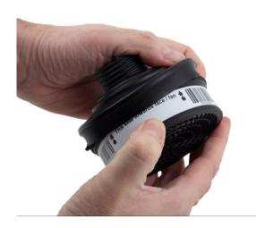
2.1 Fit the filter/combined filter in the filter adapter so that the arrows on the filter point towards the user's face. Carefully check that the edge of the filter is in the internal groove of the filter mounting all around.
