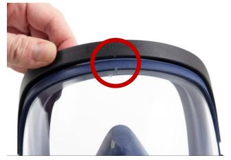
**6.6** Prise the upper frame half, making sure that the center markings are in line.
