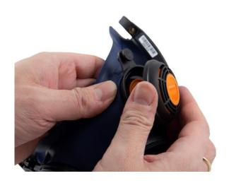
**8.1** The exhalation membranes are mounted on a fixed dowel on the inside of the valve covers on each side of the outer mask. The covers should be changed whenever the membranes are changed. Snap the valve covers off the valve seats.
