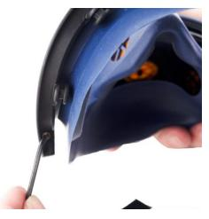
6.1 The visor is mounted in a groove running around the visor opening of the outer mask and is held in place by one upper and one lower frame half. Use a 2.5 mm Allen key to remove the two screws holding the frame halves together.
