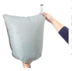
1.4 Place the equipment in the bag and grip the lower part of the bag so that the bag seals around the breathing hose. Grip the flow meter with the other hand and hold it so that the tube points vertically up from the bag.
