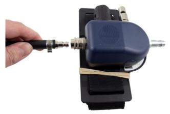
1.1 Check that the minimum flow of air through the adapter is about 150 l/min. Proceed as follows:
