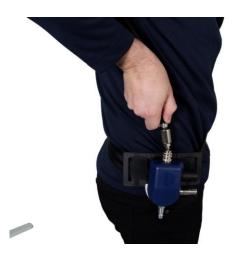
2.4 Connect the breathing hose of the compressed air attachment to the control valve outlet.
