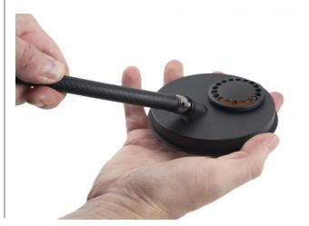
**6.4** Apply a load to the hose to check that it is firmly secured to the adapter.
