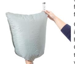
9.3 Place the head top in the flow meter bag and start the fan.
