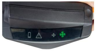
**6.4** If the button is pressed again, boosted operating status will be activated, with a flow at least 225 I/min. This is indicated by the larger green fan symbol lighting up. To revert to normal operation, press the control button once again.
