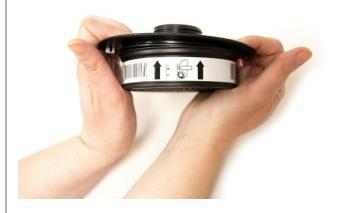
**4.3** Do not press onto the centre of the filter – it might damage the filter paper.
