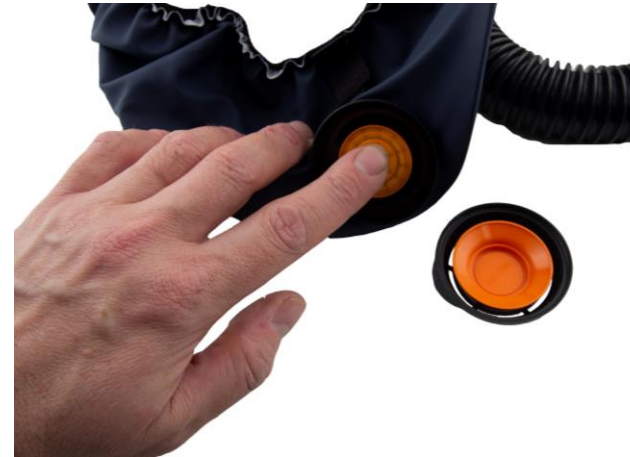
4.3 Press the new membrane onto the pin. Carefully check that the membrane is in contact with the valve seat all way round.
