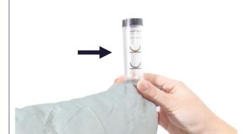
2.2 Place the head-top in the flow meter and start the fan unit. Grip the bag to seal around the breathing hose. Grip the flow meter tube with the other hand, the tube will point upwards from the bag
