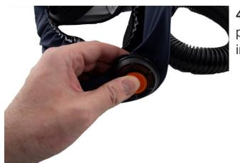
**4.4** Press the valve cover into place. A clicking sound indicates that it is in place.
