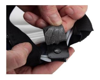
**5.1** Pick away one end of the sweatband so that it is removed together with the tape Pull sweatband off.
