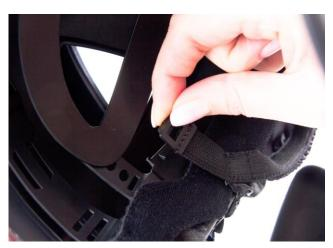
**8.1** Release the face seal hooks from the head harness.
