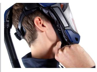
**4.3** Insert a finger between your chin and the face seal and run the finger along the contact surface of the face seal all the way round to check that it fits well against the face.
