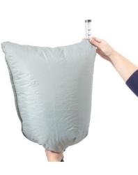
**2.2** Place the head-top in the flow meter and start the fan unit. Grip the bag to seal around the breathing hose. Grip the flow meter tube with the other hand, the tube will point upwards from the bag
