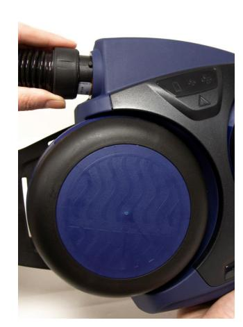
**1.2** Connect the hose from the face shield and turn clockwise about 1/8 turn
