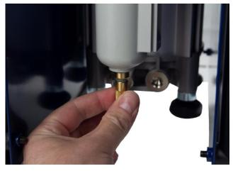
**4.1** Shut of the air inlet. Turn the pre-collector at the bottom of the drain bowl to depressurise the filter.
