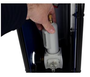
**4.2** Remove the drain bowl. Press it downward and twist anti-clockwise (bayonet mounting). Wash the bowl in hot water (not solvent) at a maximum of 60 °C.
