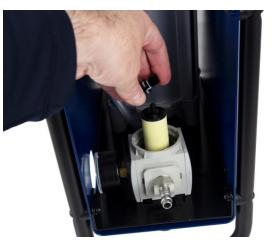
**4.3** Blow the parts clean with compressed air. Check that the drain outlet is not obstructed.
