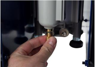
**2.1** Shut off the air inlet. Turn the pre-collector at the bottom of the drain bowl to depressurise the filter.
