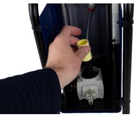
**3.4** Blow the parts clean with compressed air. Check that the drain outlet is not obstructed.
