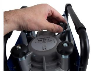
**2.3** Unscrew the knobs of the filter housing and remove the lid.
