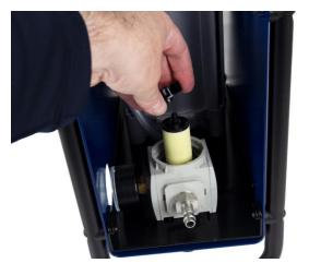
**3.3** Remove the pre-collector element by turning it anticlockwise.
