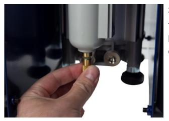
**3.1** Shut off the air inlet. Turn the pre-collector at the bottom of the drain bowl to depressurise the filter.
