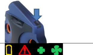
The fan will start and perform a self-test. During the test, the display symbols will light up, the alarm will sound, and the vibrator will buzz twice.
