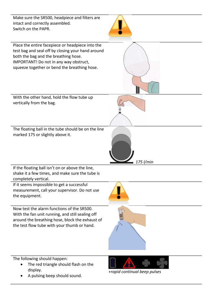
When the air block is released, all alarms should stop after about 15 seconds.
